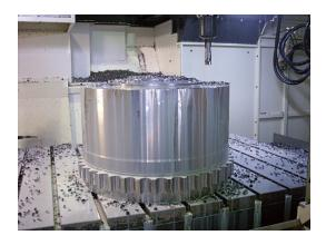
$\label{eq:machining hubTCB} \textbf{Machining hubTCB$^{\$}$-HD-10200}.$
