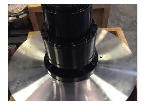
Gear coupling with brake disc.
