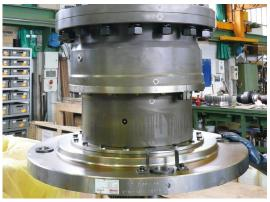
Shear pin type gear coupling
