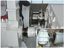
Barrel and gear coupling with brake disc.
