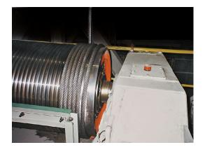
Hoisting mechanism in a steel picking line.
