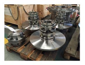
Disc pack configuration with brake disc.
